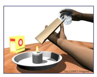
7. "Pour" the gas in the beaker or jar down the funnel. The flame will go out in a second or two. (Only pour gas)
